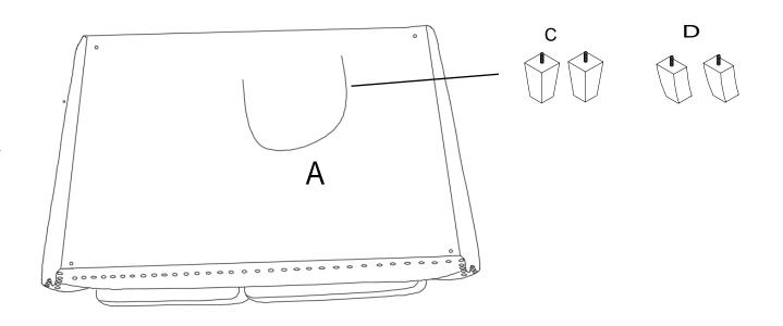
Step#2 Align the legs to the pre-drilled holes as shown in drawing, rotate to tighten it.
