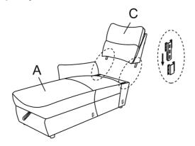
Step #5 Align and connect metal hooks to assemble the sectional.
