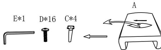
Step 2: Align the legs onto the pre-drilled holes at the bottom of unit, insert bolts then tighten with Allen key.
