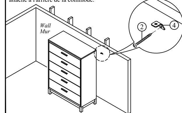
Step 3: Place the chest into position so both mounting brackets are vertically in line. Lace the end of the restraint strap through the bigger hole on each bracket. Bring both ends together and slide the flat end through the locking end and draw it through until all slack is removed. Please make sure that the strap is securely laced and locked.
