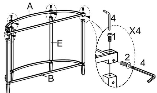
**DO NOT TIGHTEN BOLTS UNTIL COMPLETELY ASSEMBLED.**
