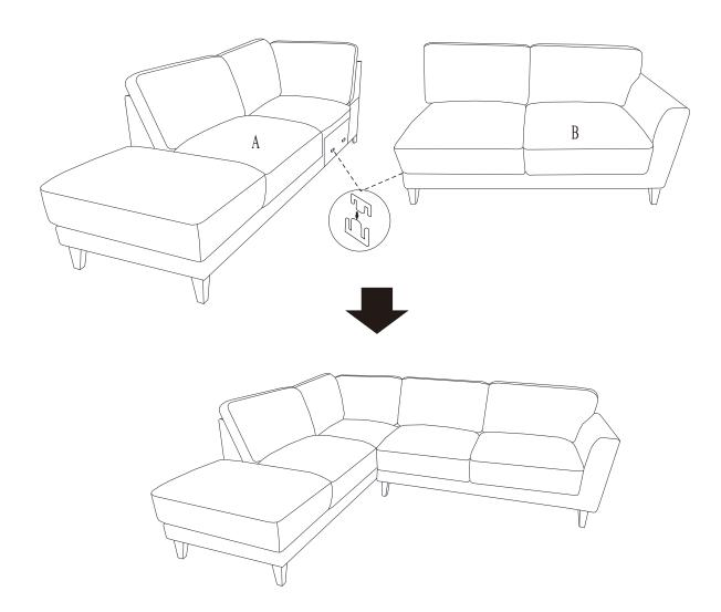
Align the female brackets at the back onto the male bracket at the seat, insert back rest to the seat then push to the end and make sure it is fixed in position securely.
