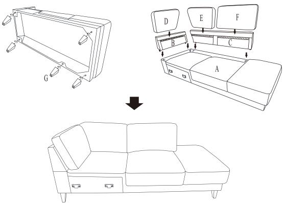
Align the female brackets at the back onto the male bracket at the seat, insert back rest to the seat then push to the end and make sure it is fixed in position securely.
