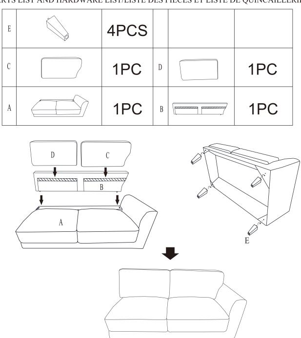
Align the female brackets at the back onto the male bracket at the seat, insert back rest to the seat then push to the end and make sure it is fixed in position securely.
