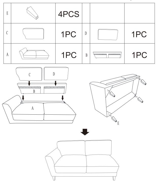
Align the female brackets at the back onto the male bracket at the seat, insert back rest to the seat then push to the end and make sure it is fixed in position securely.
