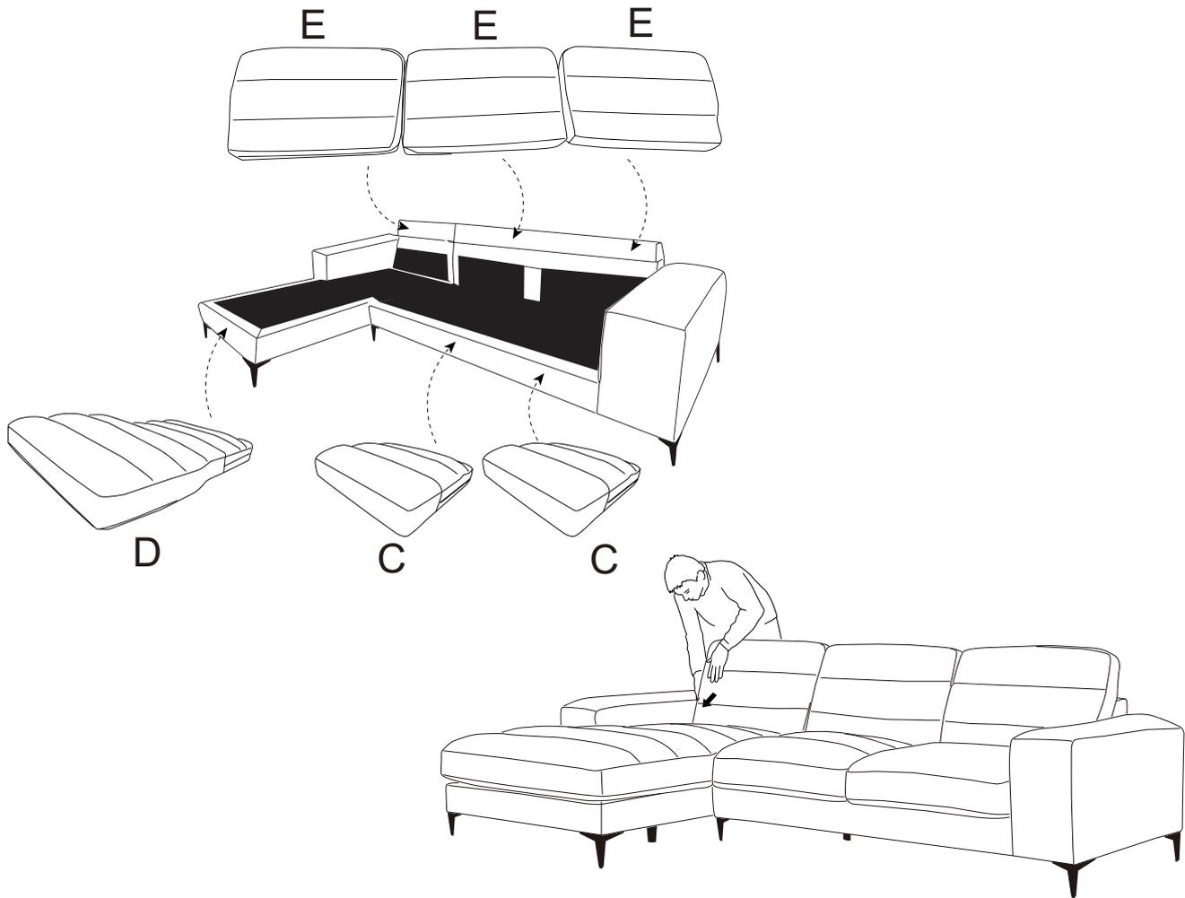
**DO NOT TIGHTEN BOLTS UNTIL COMPLETELY ASSEMBLED -- NE PAS SERRER LES BOULONS JUSQU'À CE QUE LE MONTAGE SOIT COMPLETMENT TERMINE**
