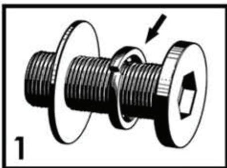
1 Before attaching each of the screws, make sure that the **smaller lock washer is between** the larger washer and the head of the screw.
