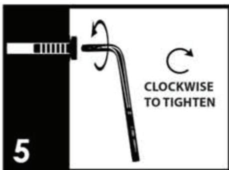
5 Finally, make sure all parts are properly aligned then use the included **tools** to completely tighten the screws. Your furniture is now ready for use.
