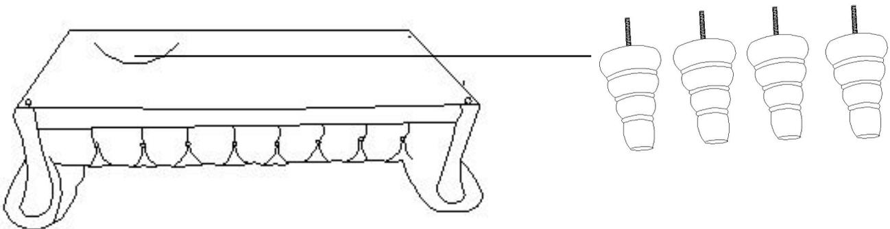
**Step#2** Align the legs to the pre-drilled holes as shown in drawing, rotate the legs in order to tighten it in secure and proper position.
