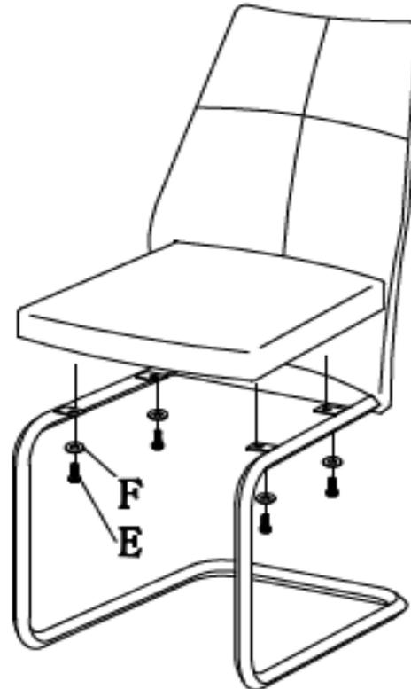
**DO NOT TIGHTEN BOLTS UNTIL COMPLETELY ASSEMBLED.**
