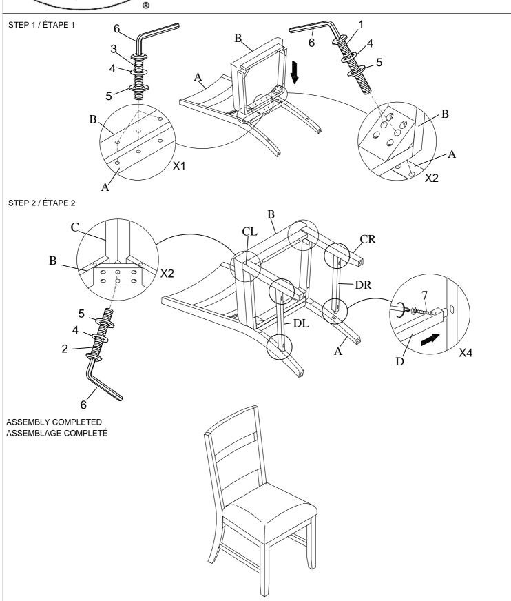
DO NOT TIGHTEN SCREWS AND BOLTS UNTIL COMPLETELY ASSEMBLED.
