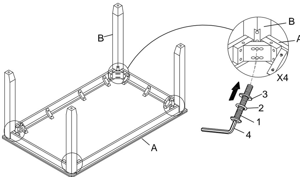
DO NOT TIGHTEN SCREWS AND BOLTS UNTIL COMPLETELY ASSEMBLED.
