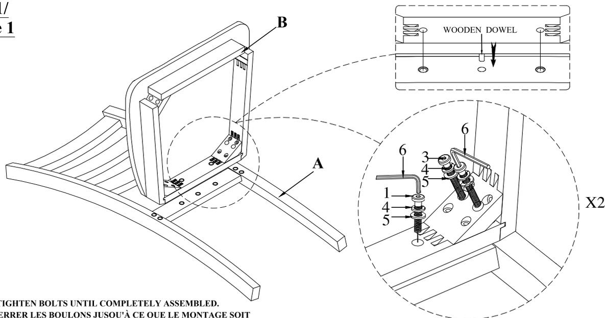
DO NOT TIGHTEN BOLTS UNTIL COMPLETELY ASSEMBLED.
