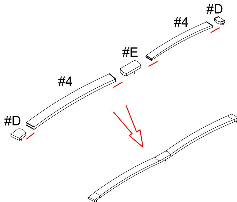
**Do not tighten screws until completely assembled. /
