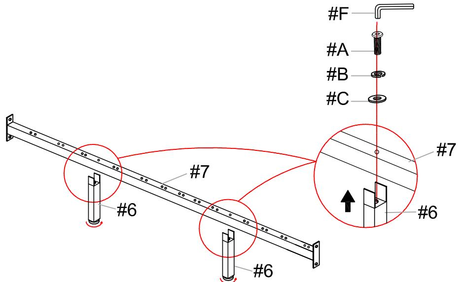
**Do not tighten screws until completely assembled. /
