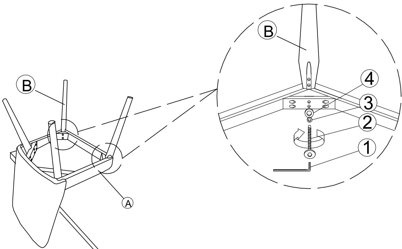
DO NOT TIGHTEN BOLTS UNTIL COMPLETELY ASSEMBLED.
