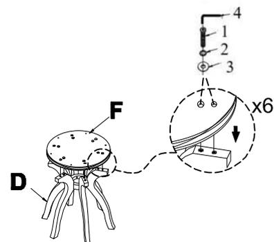
DO NOT TIGHTEN BOLTS UNTIL COMPLETELY ASSEMBLED.
