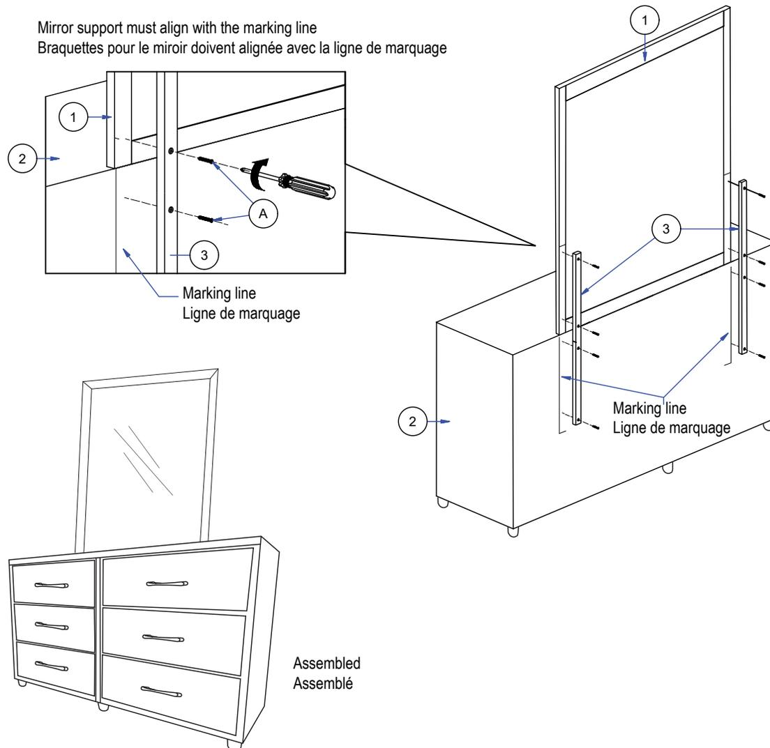
**DO NOT TIGHTEN BOLTS UNTIL COMPLETELY ASSEMBLED.**
