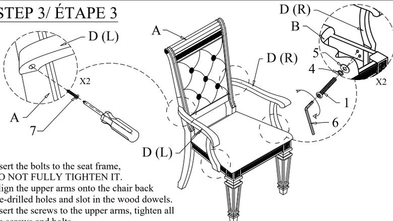
Insert the bolts to the seat frame, DO NOT FULLY TIGHTEN IT.
