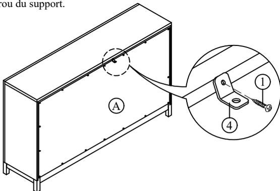
Step 2: Attached the second bracket securely to the wall using the provided longer 50mm screw, through the smaller hole of the bracket. Please attach the second bracket to the wall 2 inches lower than the first bracket that was attached to the back of the dresser.
