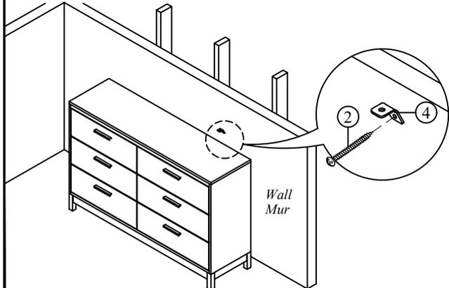
Step 3: Place the dresser into position so both mounting brackets are vertically in line. Lace the end of the restraint strap through the bigger hole on each bracket. Bring both ends together and slide the flat end through the locking end and draw it through until all slack is removed. Please make sure that the strap is securely laced and locked.
