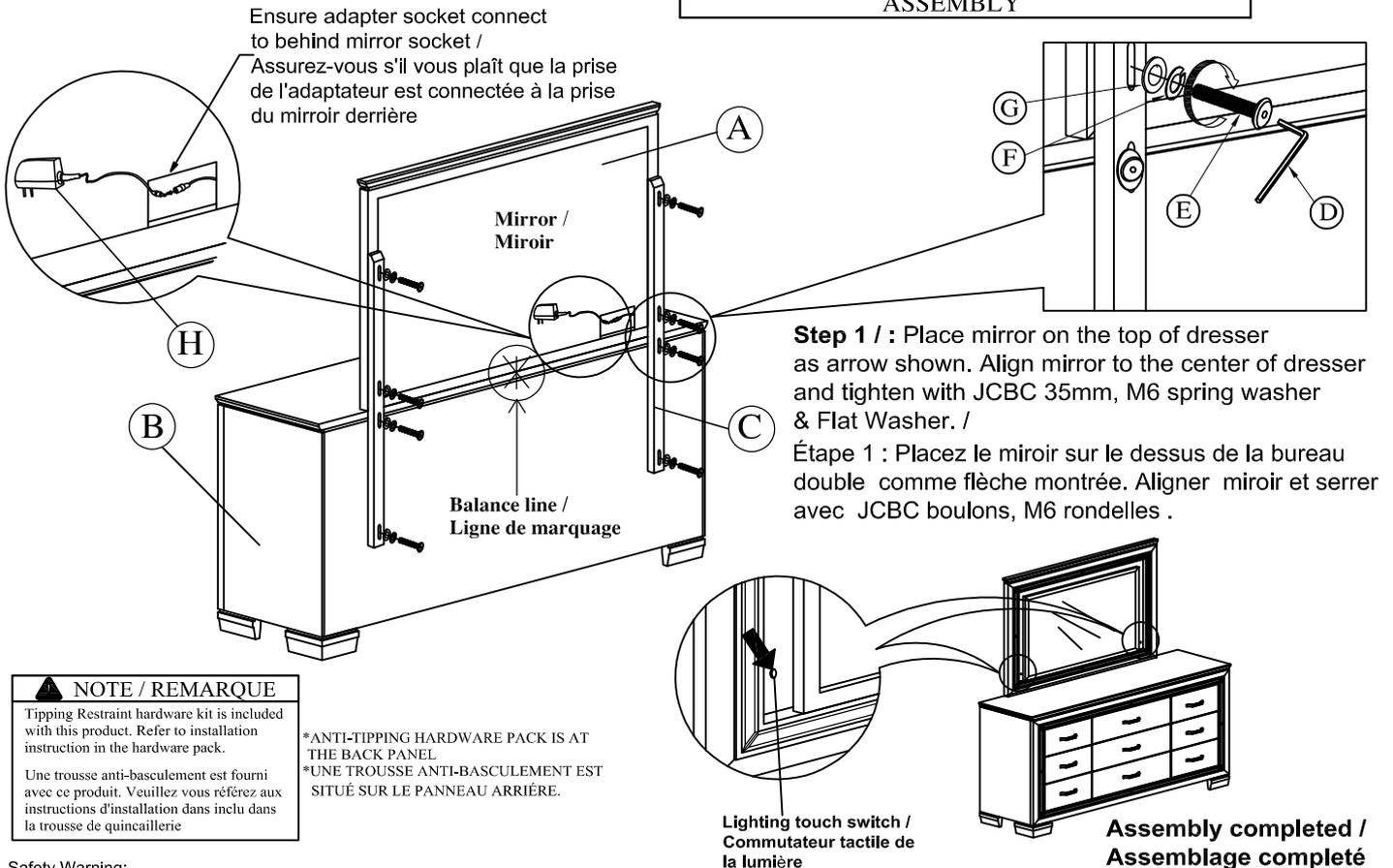
**Step 1 :** Place mirror on the top of dresser as arrow shown. Align mirror to the center of dresser and tighten with JCBC 35mm, M6 spring washer & Flat Washer. /
