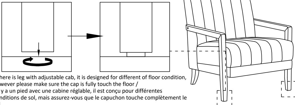
\*There is leg with adjustable cab, it is designed for different of floor condition, however please make sure the cap is fully touch the floor /
