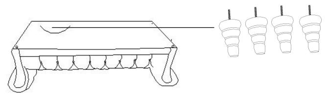
**Step#2** Align the legs to the pre-drilled holes as shown in drawing, rotate the legs in order to tighten it in secure and proper position.
