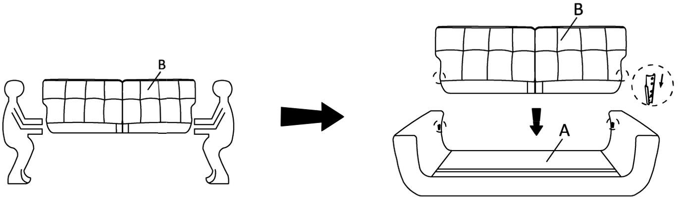
**Step #2** Please lay down the back rest and take out legs and hardware for assembly. Align and insert the bolts go through the seat, tighten with Allen key .
