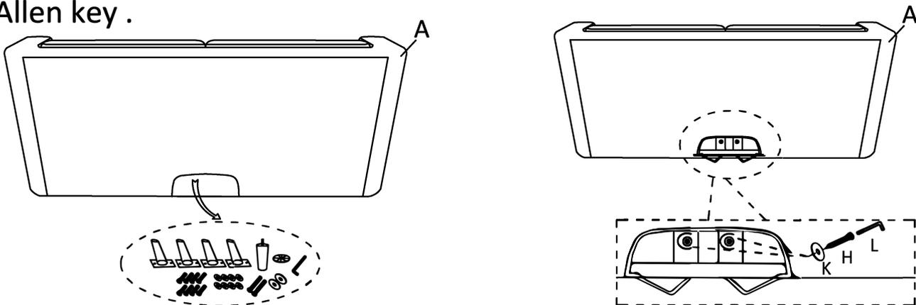
**Step #3** Align the legs to the pre-drilled holes , insert the bolts then tighten with Allen key.
