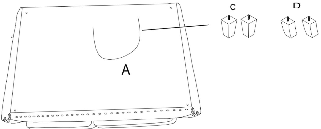
**Step#2** Align the legs to the pre-drilled holes as shown in drawing, rotate to tighten it.
