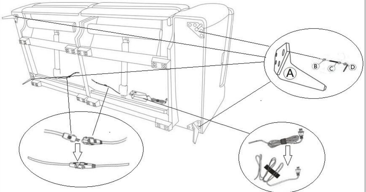
Connect two wires on motors.
