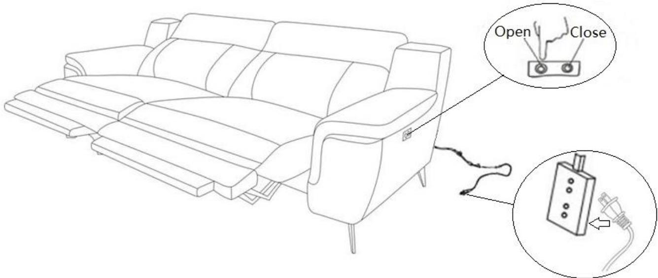
Put in to outlet to operate the unit.
